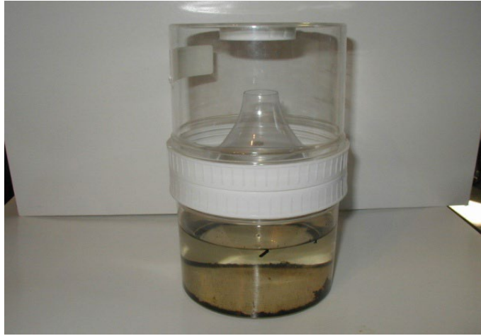
Figure 4 - Mosquito Rearing Chamber; used to allow larvae to mature into adult mosquitoes which can then be identified.
