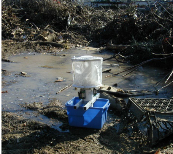
Figure 6 - The gravid trap imitates the stagnant water scenario the mosquito instinctively seeks to lay eggs
