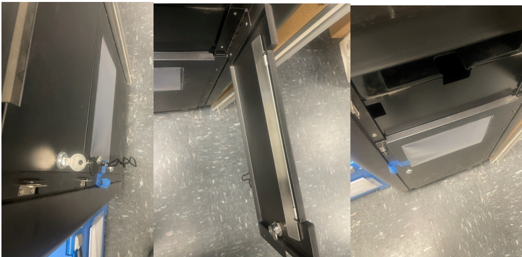
Emergency Door on DS200
