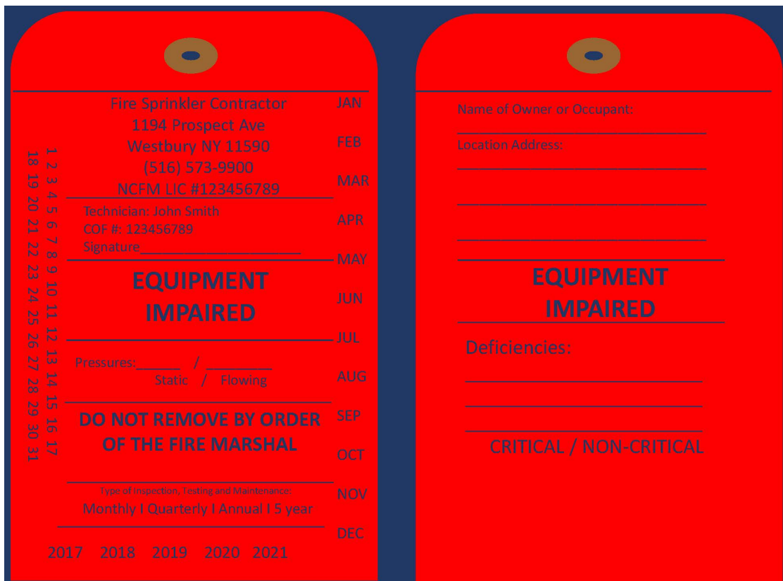
Figure 1.3: A sample of a correct ITM tag for a compliant system with equipment impairments.
