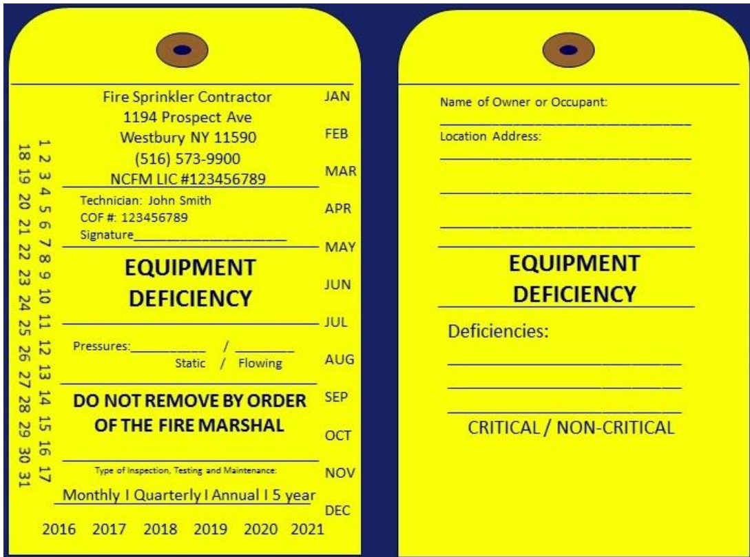
Figure 1.2: A sample of a correct ITM tag for a compliant system with equipment deficiencies.
