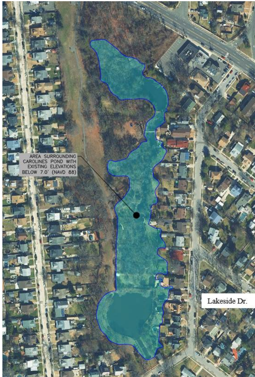
Figure III-11. Inundation Map Showing Approximate Flooding Limits at A Surface Water Elevation of 7.0' (NAVD88)
