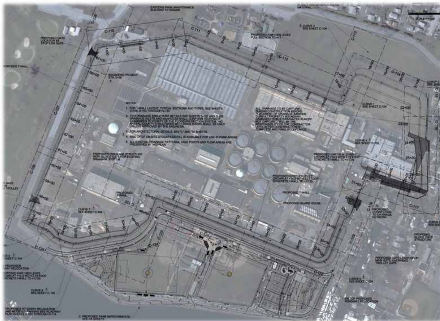
FIGURE C PROPOSED ALTERNATIVE – PERIMETER FLOOD PROTECTION BERM AND FLOOD WALL PROPOSED SITE LAYOUT
