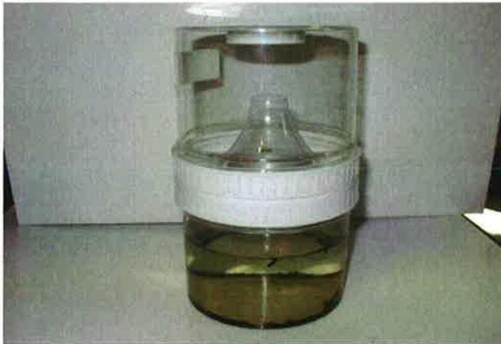
Mosquito Rearing Chamber; used to allow larvae to mature into adult mosquitoes which can then be identified.
