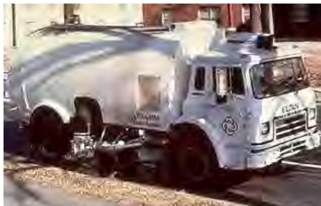
A street sweeper cleans up pollutants and sediments on the street to reduce the amount of pollutants entering receiving waters
