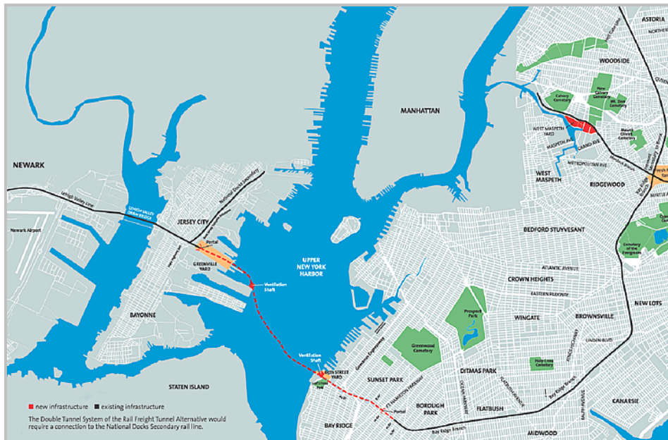
Figure 4-3 Proposed Cross Harbor Freight Tunnel
